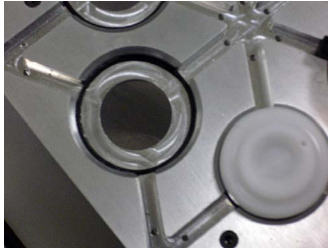
Figure 10: Nest on parts courier with compliant rubber material.
