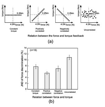
Fig. 3. (a) The experimental manipulation of the force/torque relation in the stimuli. (b) Mean JND of force discrimination as a function of the force/torque relation. Error bars represent  $\pm 1$  standard error.
