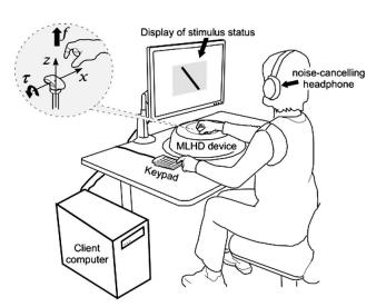
Fig. 2. Schematic illustration of the experimental setup (see text for details).
