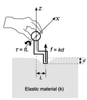
Fig. 1. Force and torque feedback produced by the tool interacting with soft tissue. Rotation is centered in the handle and about the *x*-axis. L, d, k, f, and  $\tau$  denote moment arm length, amount of deformation, stiffness, resisting force, and torque, respectively.
