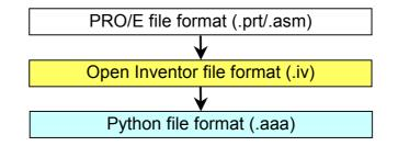
Figure 10: Conversion of part files
