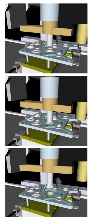
Figure 18: Pickup operation of the retainer ring #3
