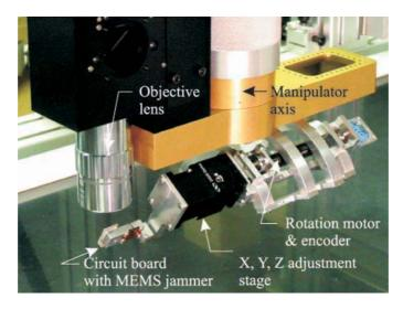
Figure 27: New end effector with attached effector mechanism
