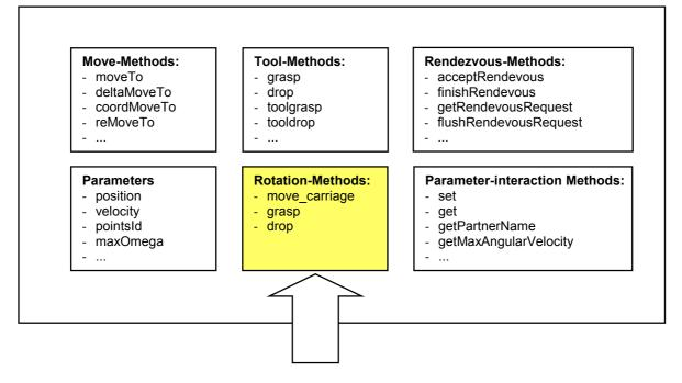
*Figure 29: Class FoProgManipulatorInterface and additional Methods for ZY-VEX project*
