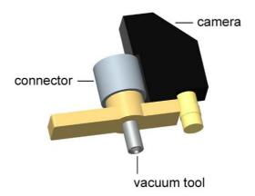
*Figure 15:* New end effector with attached OSTI vacuum tool
