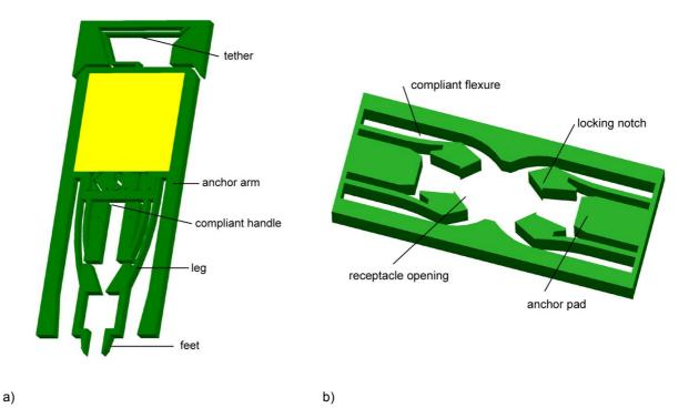
Figure 23: a) Tethered micro mirror, b) Socket
