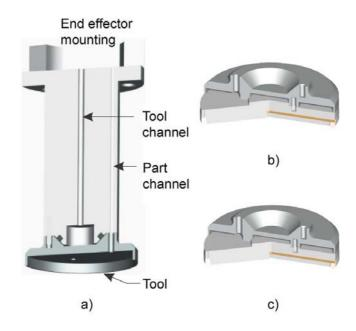
*Figure 17: a)* OSTI vacuum tool, b)+c) retainer ring tools (sections)
