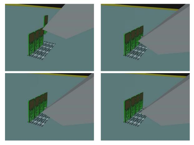
*Figure 32: Placing and fixing of a micro mirror*
