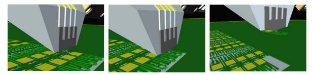
Figure 31: Detach and pick up of a micro mirror
