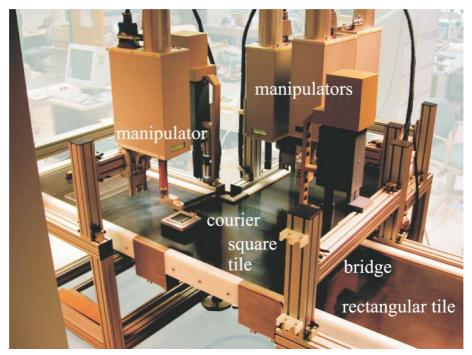
Figure 1: T-shaped Minifactory at MSL
